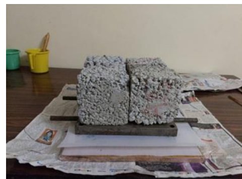
(b) Laminates curing under pressure
