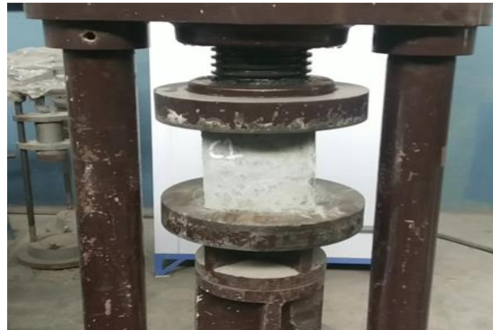
Fig 3 Compressive test of cube specimen
