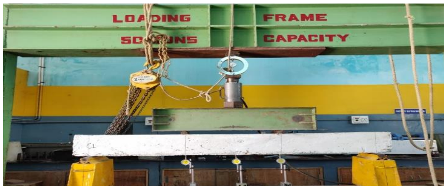
Fig 5 Experimental setup of beam
