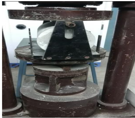
Fig 4 Split Tensile test of cylindrical specimen
