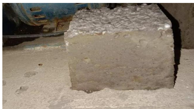
Fig 2.1: Concrete block made by fly ash and thermocol
