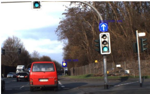
Fig 6.5: Image after traffic sign has been detected
