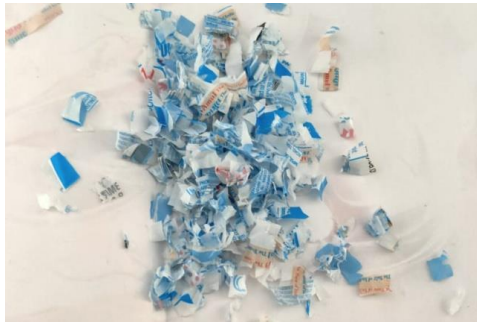
Fig 2.1 : Lime treated polyethylene strips
