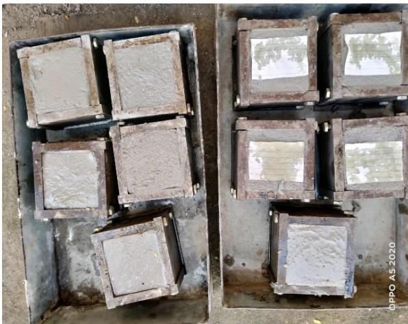
Fig -2: Casting of mortar cubes
