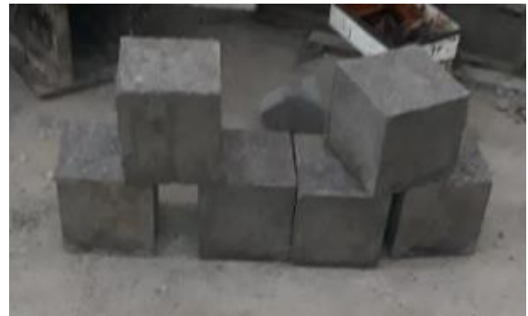
Fig.4: After 24 hours the cubes are ready to be putted in curing tank
