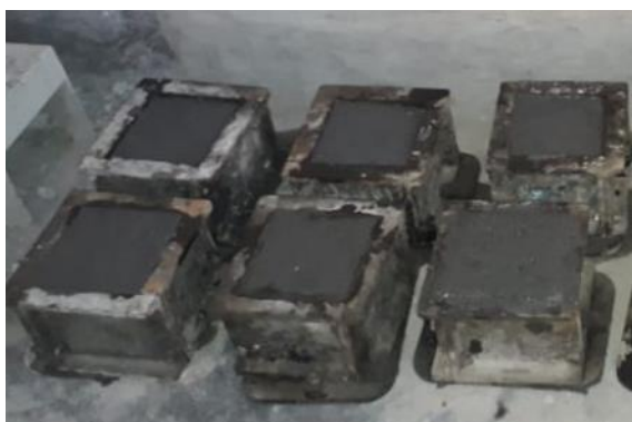
Fig.3: Casting of Cubes
