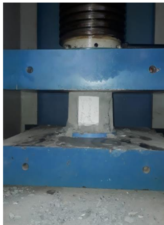
Fig.6: Cube samples after completion of test with visible cracks
