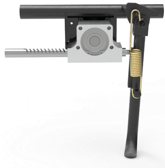
Fig -11: Automatic side stand at parked position.
