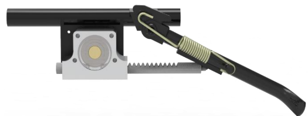
Fig -12: Automatic system pushing the side stand.
