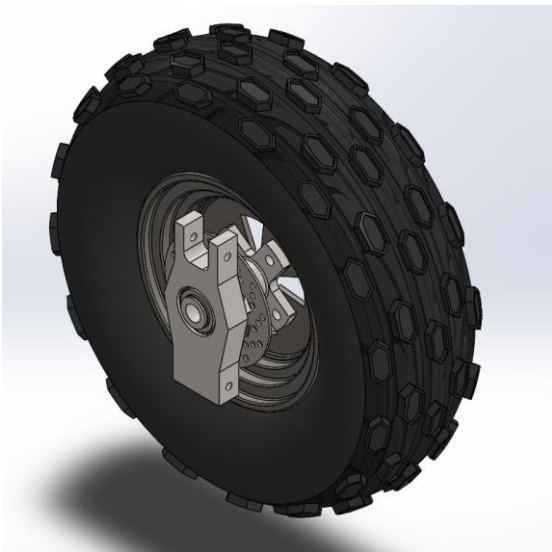
Fig 9.2: Complete Rear Wheel Assembly (CAD)
