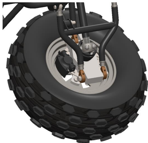
Fig 9.4: Rear Wheel Assembly with A-Arms (CAD)
