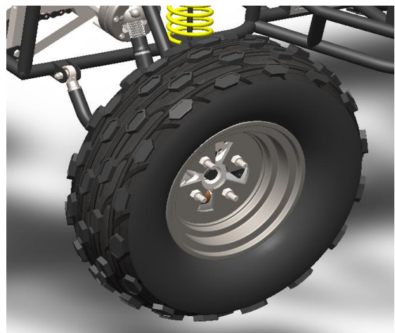
Fig 9.5: Completely Attached Rear Wheel Assembly (CAD)
