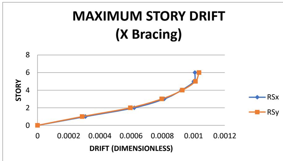
Figure.5 Maximum Story Drift (X-Bracing)
