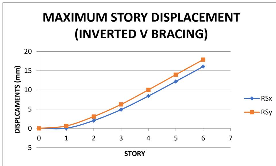
Figure 8. Maximum Story Displacement (Inverted V Bracing)
