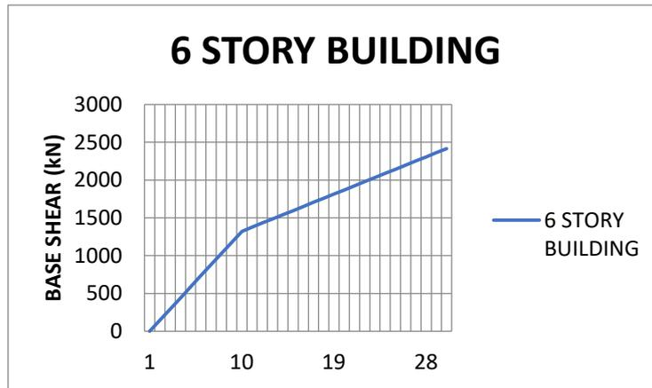
Figure 4. Monotonic Pushover Curve (Base shear vs story drift)
