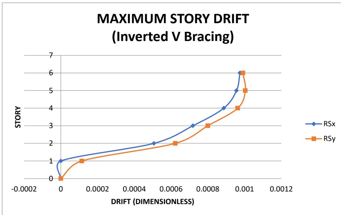
Figure.6 Maximum Story Drift (Inverted V Bracing)
