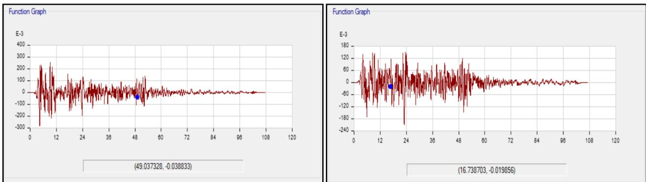
Figure.2 Ground motions of Imperial Valley : In X-direction(left) & In Y-direction(right)
