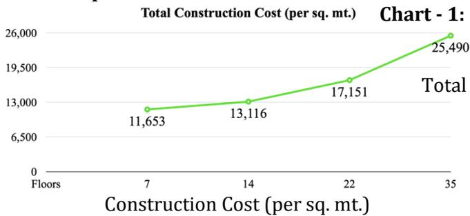
The total construction cost per square feet of 7, 14, & 22 floors is compared to that of 35 floors. The total construction cost per square feet increases by 119%, 94% & 49% for 35 floors compared to 7 floors, 14 floors & 22 floors respectively.
