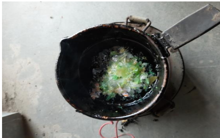
Figure 6: Heating of Bitumen and Mixing of Waste plastic
