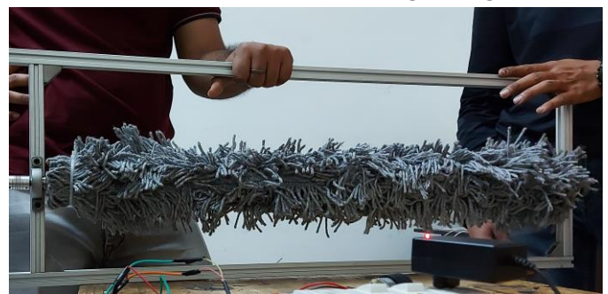
Figure -2: Cleaning Assembly
