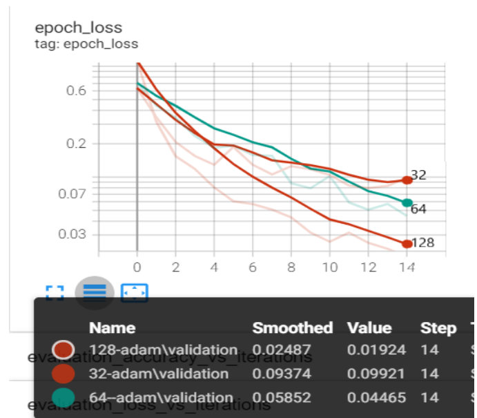
Fig 8. Validation accuracy and loss using Adam optimizer while training on different batch size
