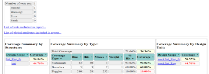
Fig -26: Code coverage report of Integer Register File without fault
