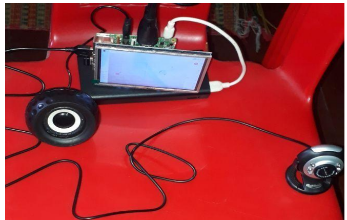
Fig -4: Raspberry Pi interfaced with webcam and speaker
