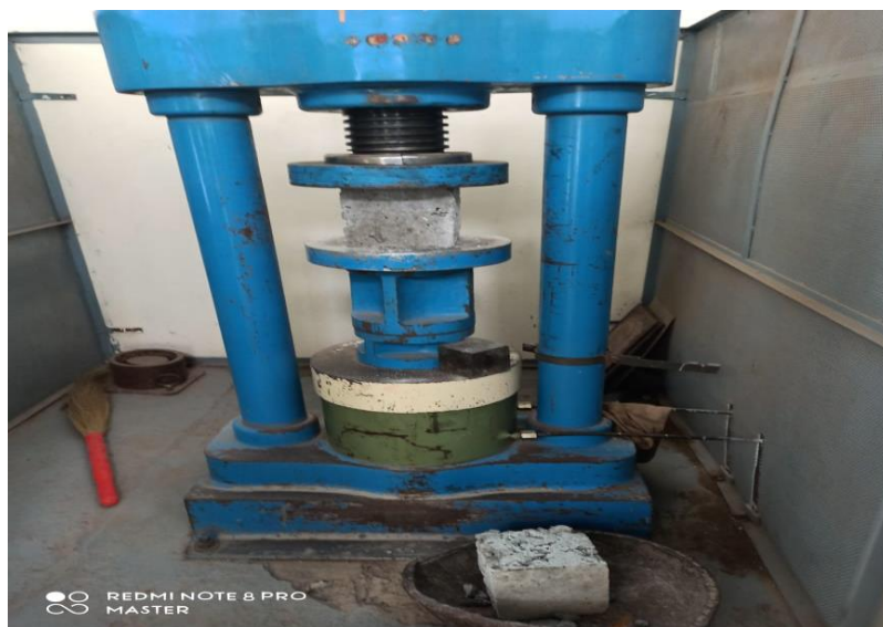
Fig 5: Compressive test on cubes
