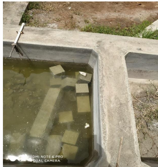
Fig 4: Curing of concrete cubes cylinders and beams
