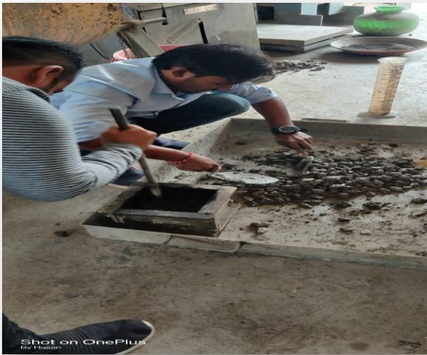
Fig 3: Tamping of concrete in mould
