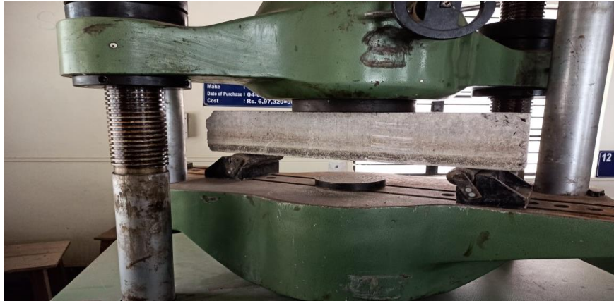
Fig 7: Flexural test on beam
