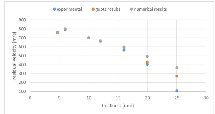
**Fig- 8:** Residual velocity of projectile function of thickness
