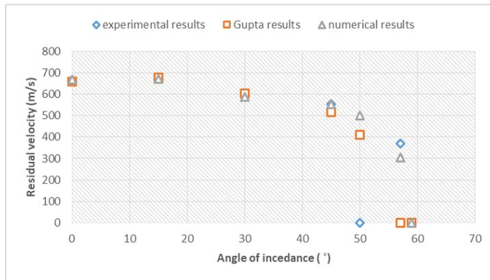
**Fig -7:** Residual velocity of projectile function of obliquity
