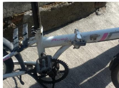
Fig -3: Folding mechanism of middle rod
