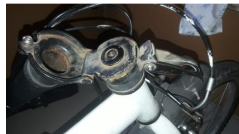
Fig -2: Unfolding mechanism of front rod
