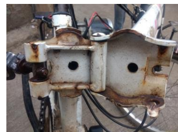
Fig -4: Unfolding mechanism of middle rod
