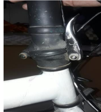
Fig -1: Folding mechanism of front rod
