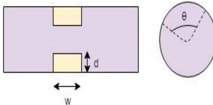
**Figure 1:** Typical Notch geometry
