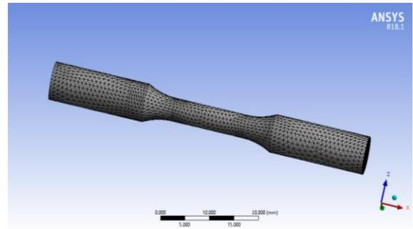
(b) Finite Element Model after meshing
