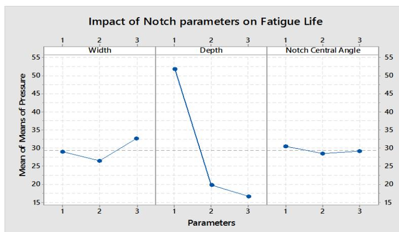
**Figure 6:** Variation of Pressure w.r.t. the parameters
