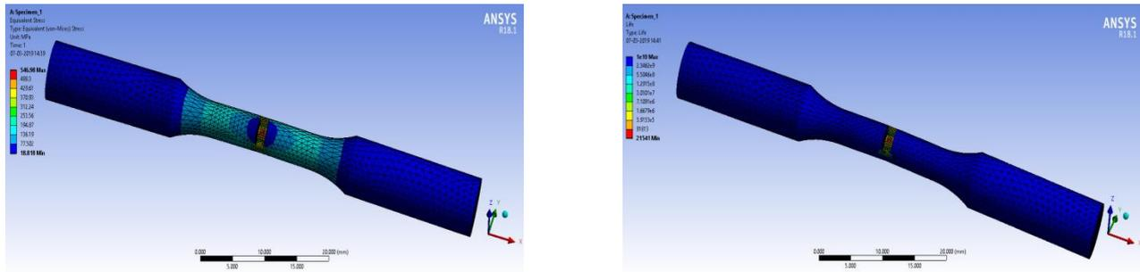
**Figure 5:** FE analysis of specimen mentioned in Run 1 (1-1-120°)
