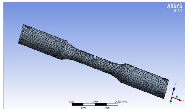
Finite element model after meshing
