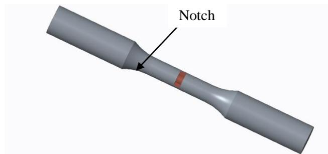
Figure 3: 3-D model of the specimen
