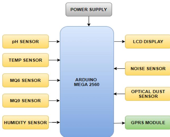
Fig -2: Transmitter section of system
