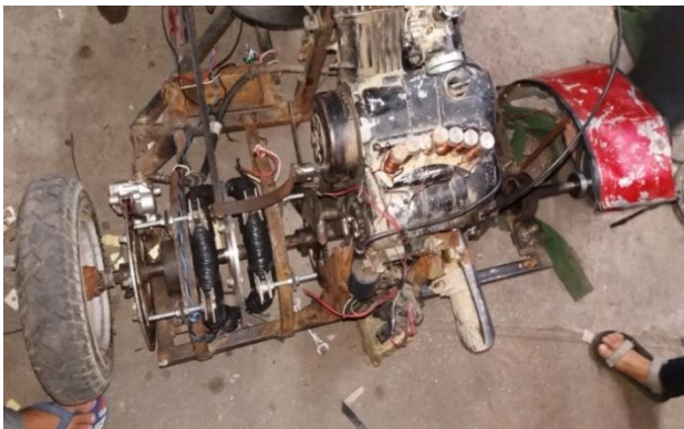
Fig-6: Installation of electromagnetic brake
