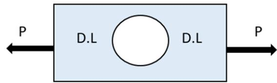
Fig-1: Image representation of panel with circular cutout
