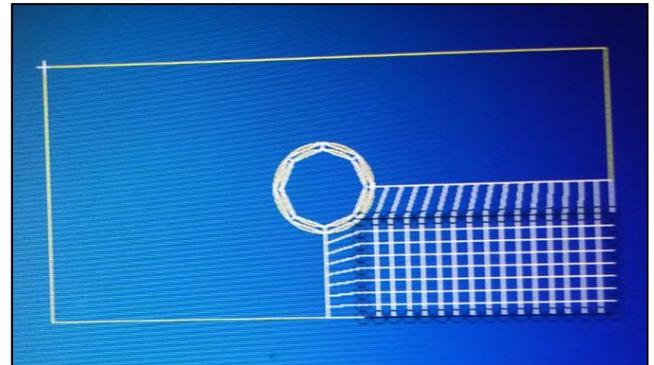
Fig-2: Meshing of one quadrant on the plate
