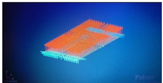
Fig-4: Loads applied to the stiffened panel
