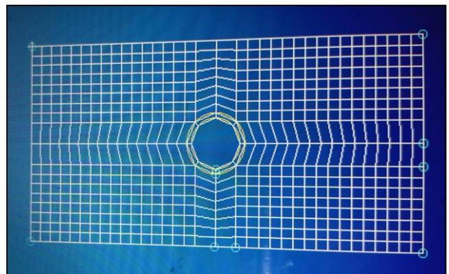
Fig-3: Mirror meshed stiffened panel and cut-out
