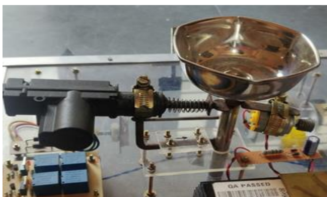
Fig. 7 Seed Planting Mechanism
