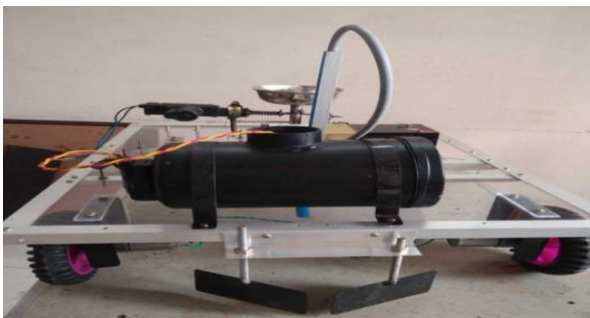
Fig. 10 Water Delivering Mechanism
