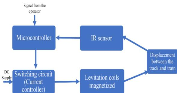
Fig -2: Block diagram for Levitation system
