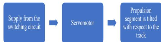
Fig -3: Block diagram for the Propulsion system
