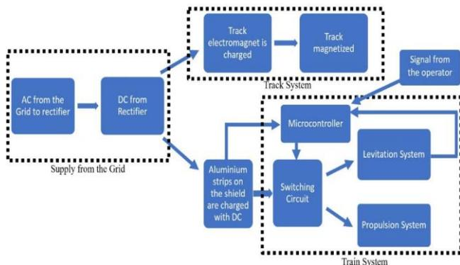
Fig -1: Main block diagram of DC Maglev train
