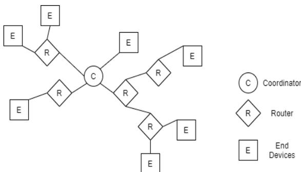
Figure 1: Mesh topology of ZigBee Devices
