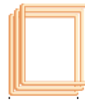
Fig-8: Rectangular Coil
