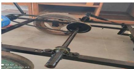
**Figure 3.1 Pulley with V-belt**
