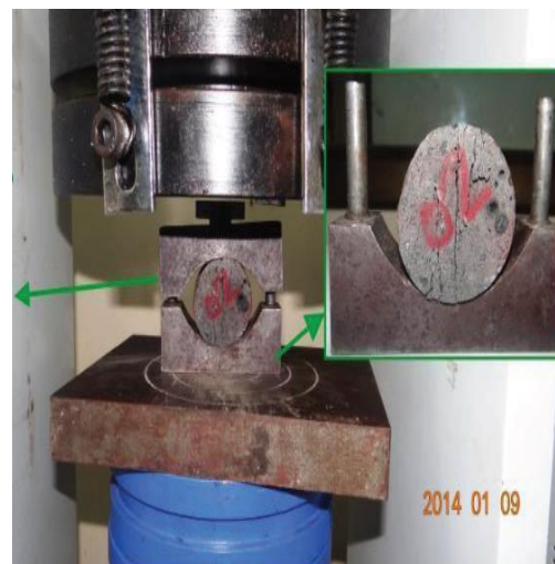
Figure 3: Tensile strength setup
