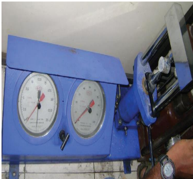
Figure 4: Point load index determination setup
