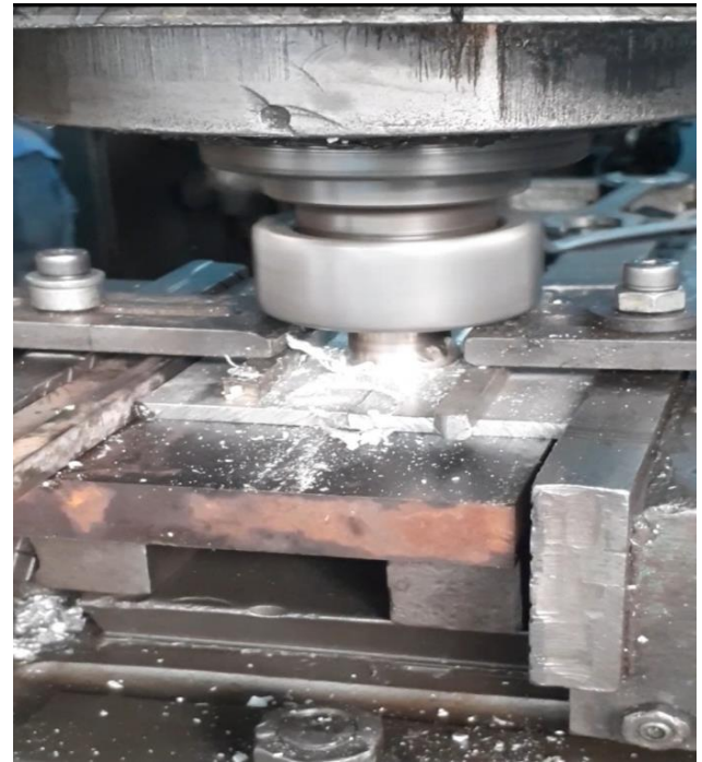
Figure 2.3: FSW process on AZ31 plates being welded with Boron powder
