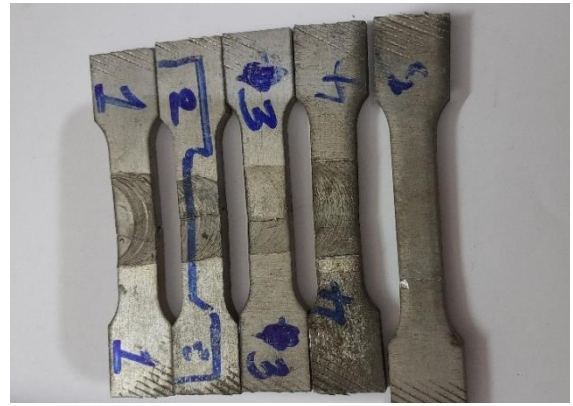
Figure 2.9: samples for tensile test after EDM wire cut machine
