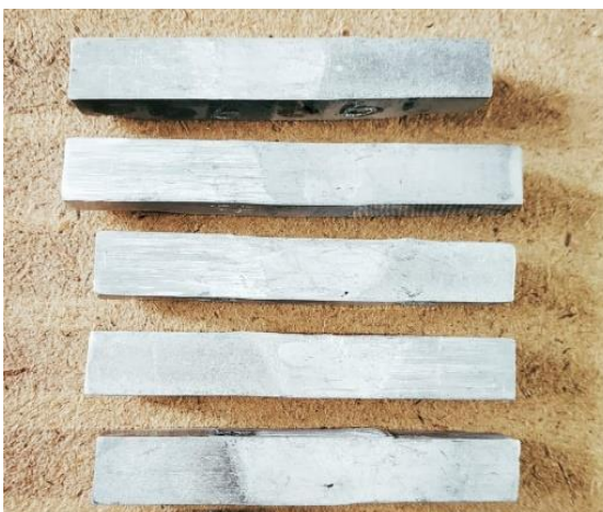
Figure 2.13: micro hardness test samples from EDM wire cut
