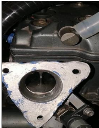
Fig 8: Manually adjusting the injector position
