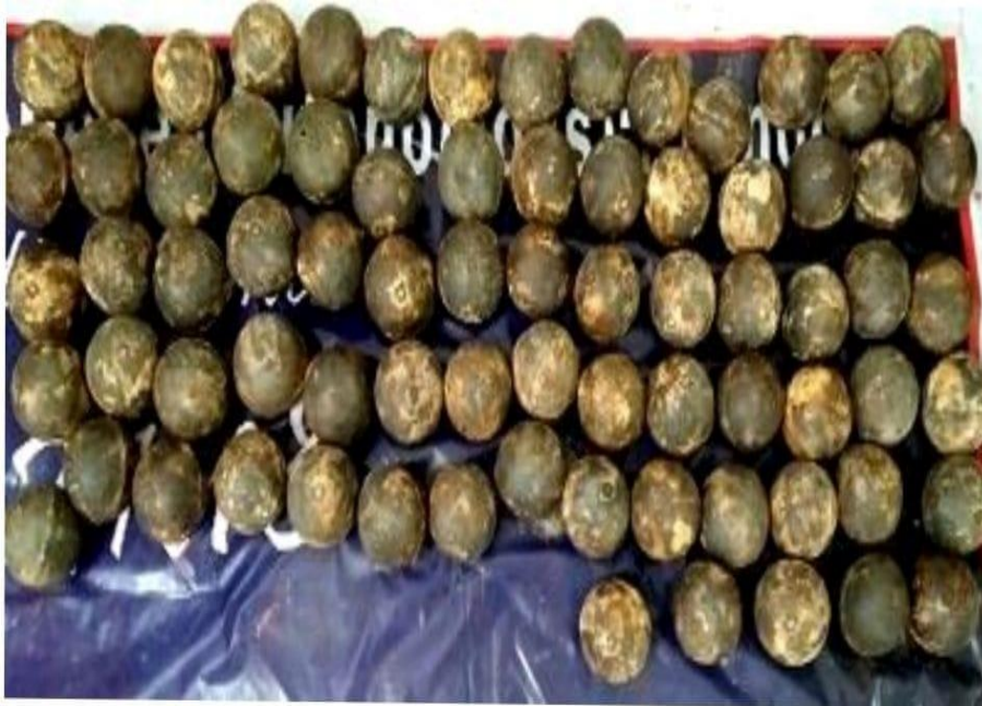
Fig 4.5 : Spherical capsules filled with the liquid PCM
