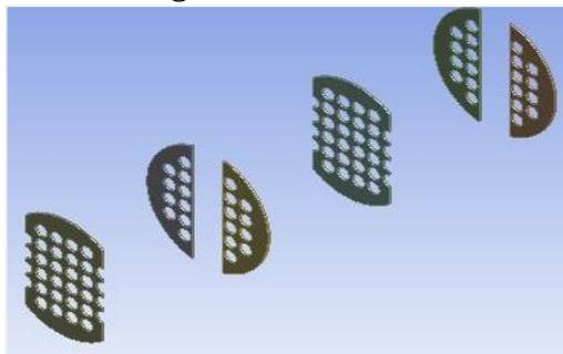
Fig.-3 DS Baffle Profile
