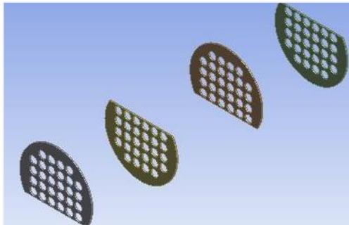
Fig.-2 SS Baffle Profile
