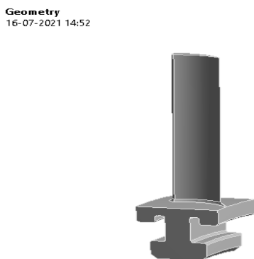
Fig -6: Isometric Industrial Gas Turbine Blade Without Holes
