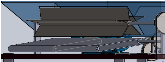
Figure 10 Conveyor position according with trolley and thrower.
