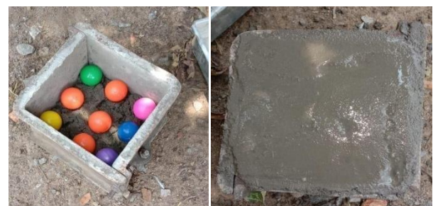
Fig -3: polyethylene balls placed in cube and finishing of cubes
