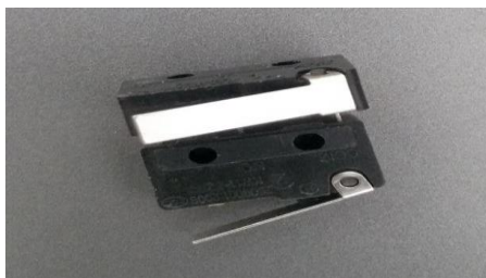
Fig-4: Limit Switch
