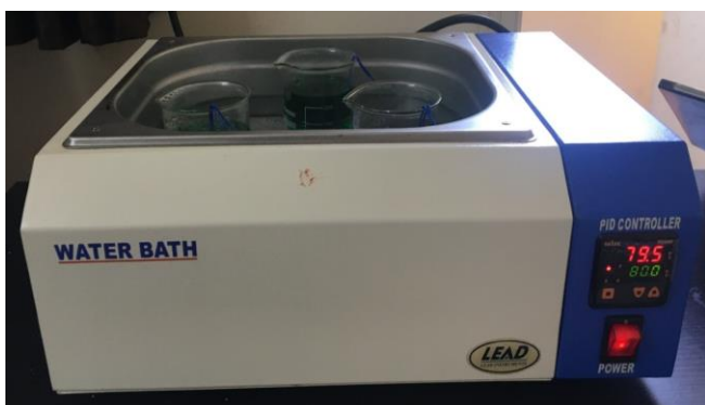
Figure 2.1: Experimental setup used for the preparation of electroless Ni-P and Ni-Cr-Mo-P coatings.
