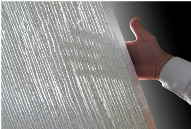
Figure-5: Light transmitting test in day light
