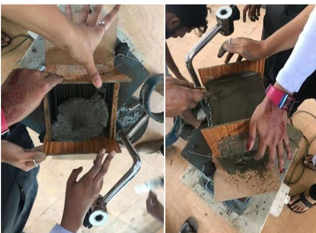
Figure-3: Stages of Pouring the Concrete
