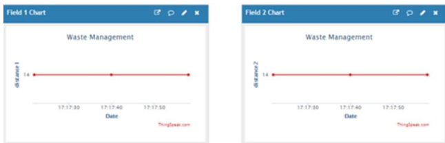
Fig -17: Graph in ThingSpeak when both the bins are empty
