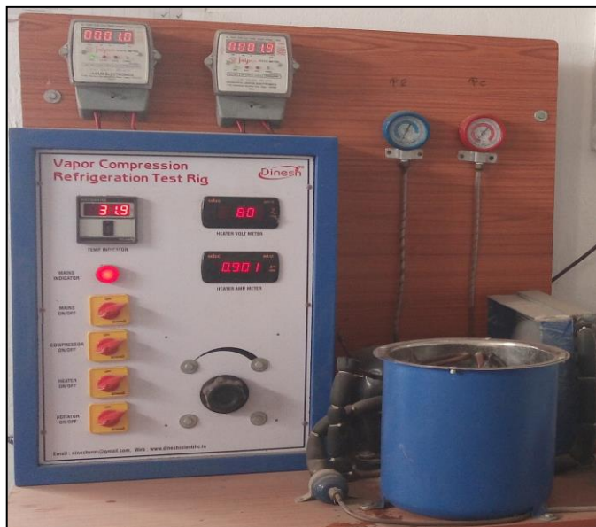
Fig -3: Test Rig of Vapour Compression Refrigeration System with PCM
