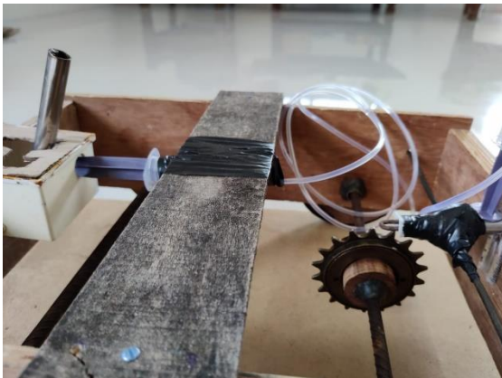
Fig -12: Disengagement of ratchet and pawl
