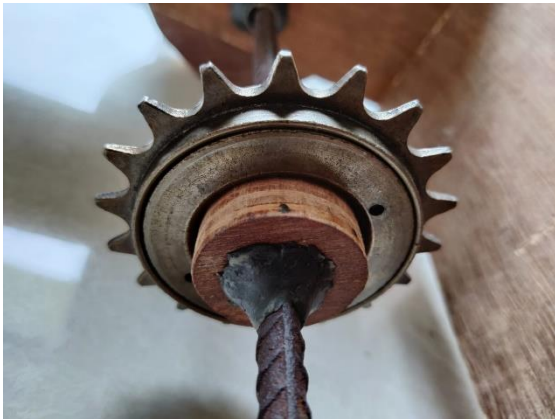
Fig -1: Freewheel used as ratchet
