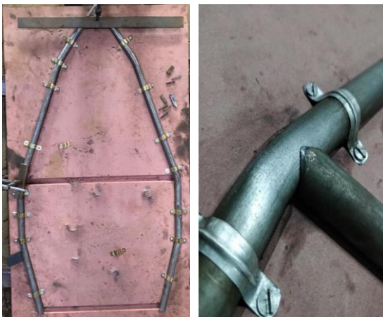
Fig -17: Fixture for holding bent Main Hoop into place
