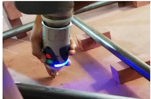
Fig -24: Setting up the coordinate system before scanning
