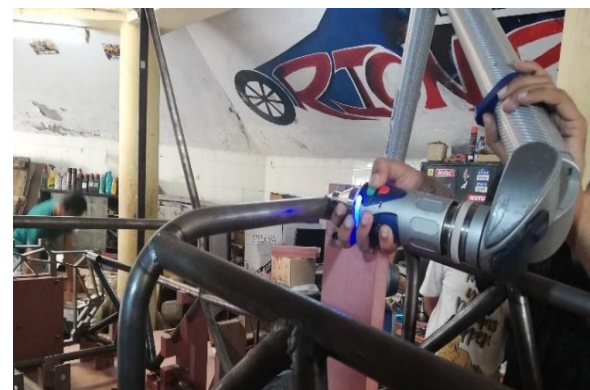
Fig -25: 3-D scanning of the chassis
