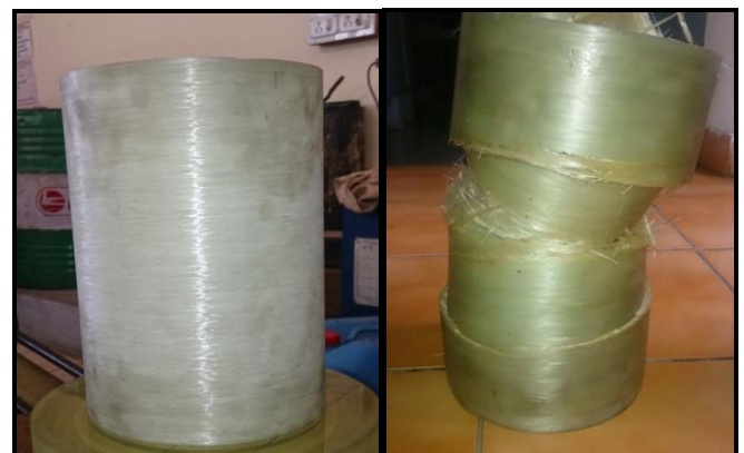
Fig 13 (a) Glass/vinyl ester cylinder before test
