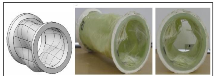
Fig 2 Buckled cylinder under external pressure
