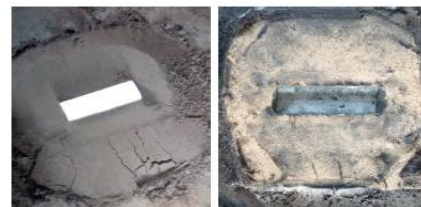
Figure 3: Fabrication Stages of The Mold.
