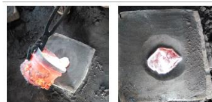
Figure 5: Pouring the Melted Aluminum Inside the Molds
