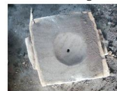
Figure 4: The Completed Mold of The Heater Block.
