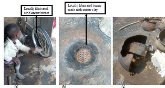
Figure 1: A Local Furnace Constructed for Melting Aluminum Scraps
