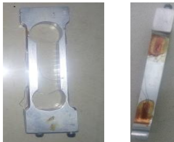
Figure 7: Shows Developed Load Cell
