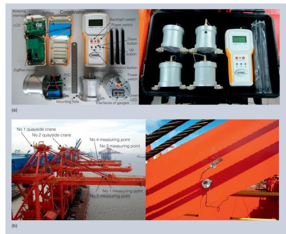
Fig. 5. 4. Wireless Sensor Network for strain monitoring on a quayside crane: a) the wireless sensor network kit for strain monitoring, b) the distribution of the WSN nodes on the level of the metallic structures
