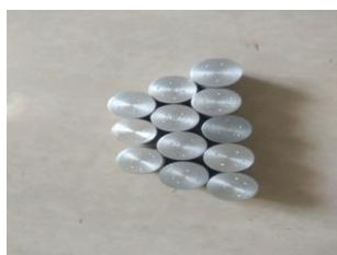
Figure 6.2 Hardness Tested Specimen
