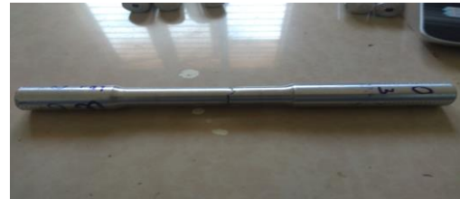
Figure 6.3 Tensile Tested Specimen
