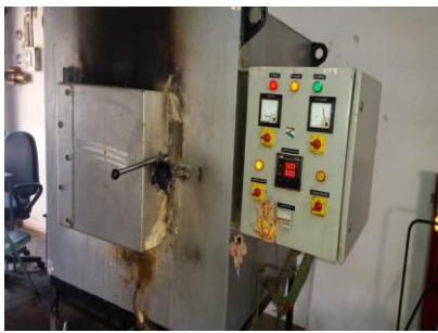
Figure 5.3 Furnace used to heating the areca sheath ash
