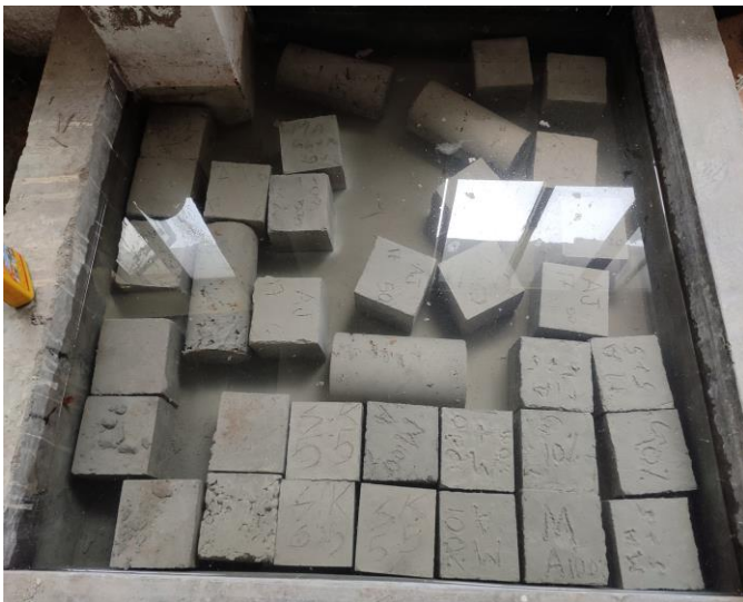
Figure 5.0: Concrete Specimens in Curing Tank
