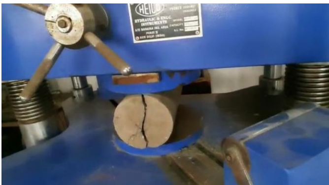
Figure 6.0: Universal Testing Machine (UTM) with a Test Specimen
