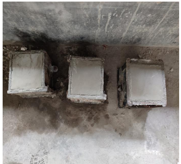
Figure 4.0: Casting of Concrete specimens
