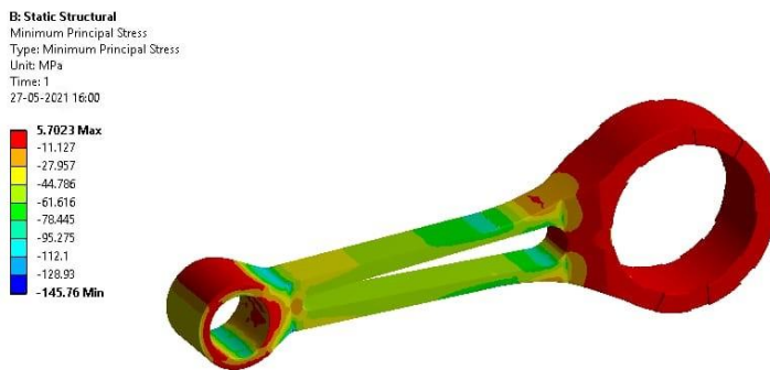
Fig - 16: Minimum principal stress is 5.7023 MPa
