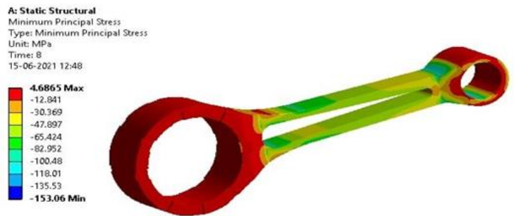
Fig - 10: Minimum principal stress is 4.6865 MPa
