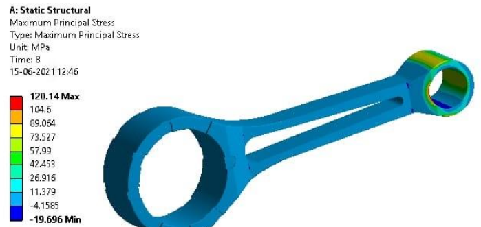
Fig - 11: Maximum principal stress is 120.14 MPa
