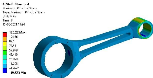
Fig - 15: Maximum principal stress is 120.22 MPa
