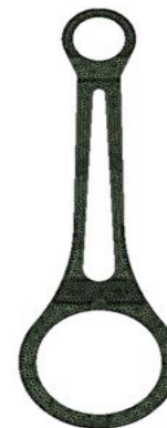
Fig - 7: Meshing connecting rod with cutout
