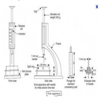
\*GRADUATED SCALE: graduated scale shall be of 40mmin length and the smallest division on the scale is 1mm.
